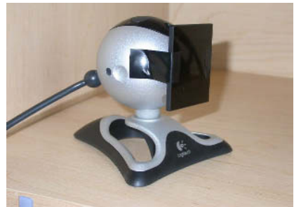
Fig. 2. One of the webcams with an IR pass filter used for a Tracking camera. Note: the camera has its IR filter removed.
