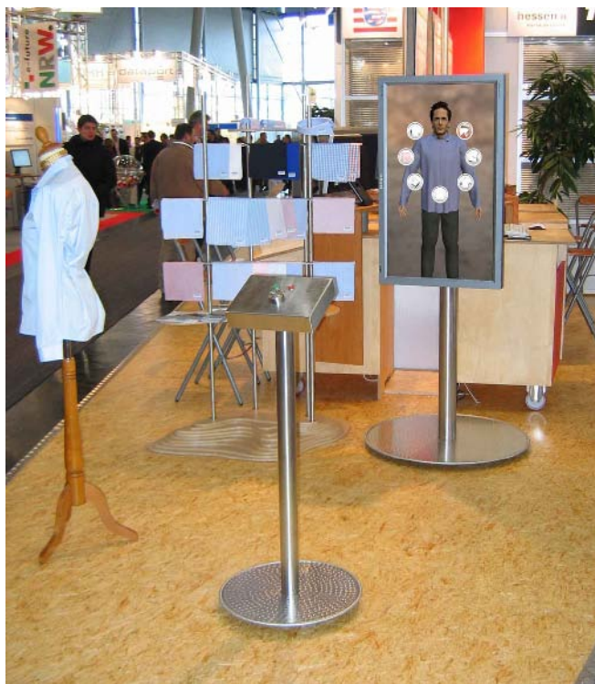
Fig. 1. IntExMa prototype: customized interaction device (middle) and 3D product visualization with GUI on top (right)
