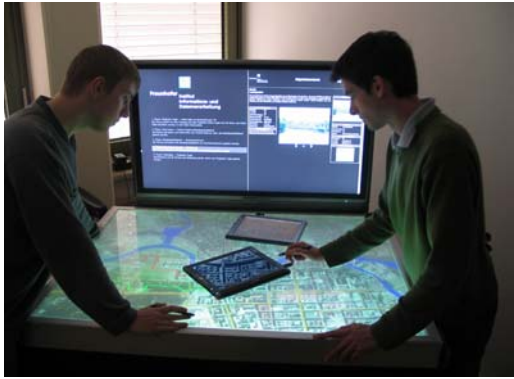
Fig. 3. The »digital map table« of Fraunhofer IITB with its horizontal table for scene overview, two Fovea-Tablets on top of this table illustrating scene details, and a vertical board displaying additional information.
