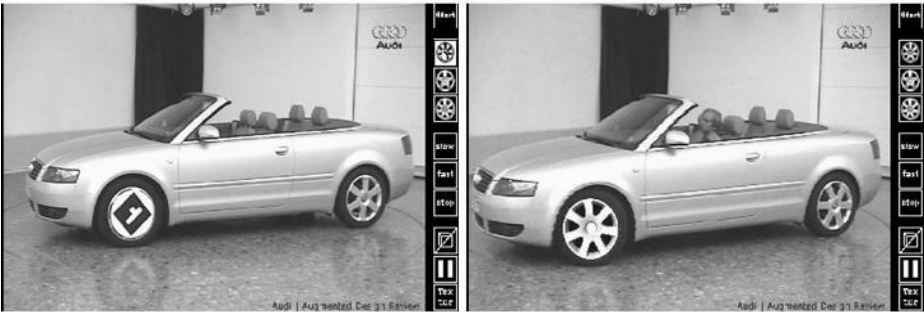
Fig. 2. Marker-based augmented reality (augmented video) applied in marketing: The video shows a car with a marker placed on the front-left felly (left). The user then selects one of the available fellies to augment the video with the virtual felly following the movement of the car in the right perspective position (right). In this way the user get a visual impression of the felly.
